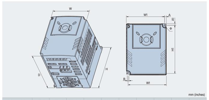
**Drive model** (kW) W (mm) W1 (mm) H1 (mm) A (mm) H (mm) D (mm) Φ B (mm) (kg) SV015IG5A-1 0.75 100 95.5 128 120 130 4.5 4.5 4.5 1.12 1.5 100 95.5 128 120 130 4.5 4.5 4.5 SV015IG5A-2 1.12 SV015IG5A-4 1.5 100 95.5 128 120 130 4.5 4.5 4.5 1.12
