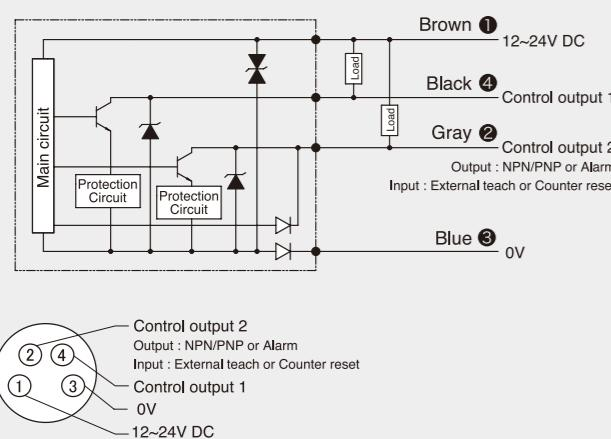
The operation of each output can be set to Light-On / Dark-On. Also, the Threshold level, Timer settings, etc. of each output can be set independently. The Analog output type (D2RF-TAN/P) provides a 4 ~ 20 mA (gray wire) analog output and a NPN (or PNP) digital output (black wire).
